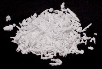
magnesium perchlorate flakes
